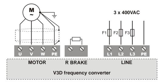
The power on the brake resistor (Pnominal /  $50 \div$  Pnominal) depends on the braking time and the duty factor. Selection guide on page 21.
