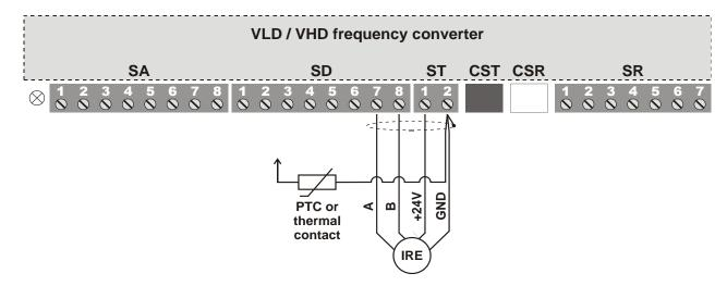
The signal device can be NPN open collector type, TTL push-pull type or an output with an output voltage of 5 to 24 V. Independently of the signal transmitter input, the further digital inputs can be operated with both negative and positive logic circuitry.
