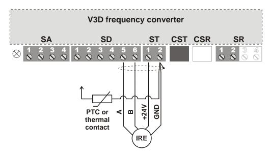
The signal device can be NPN open collector type, TTL push-pull type or an output with an output voltage of 5 to 24 V. Independently of the signal transmitter input, the further digital inputs can be operated with both negative and positive logic circuitry.
