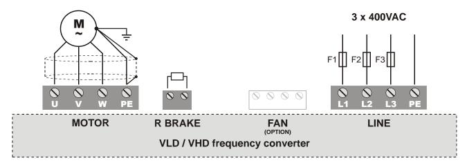
The power on the brake resistor (Pnominal / 50 ÷ Pnominal) depends on the braking time and the duty factor. Selection guide on page 21.
